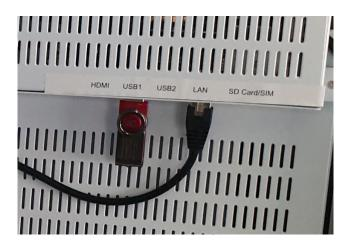
5. When the first pop up message appears, use a USB mouse to click the checkbox 'Use by default for this USB device?' and click OK (a USB mouse can be inserted into USB2).
